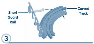
•"Snap" the short guardrails onto the curved tracks.
